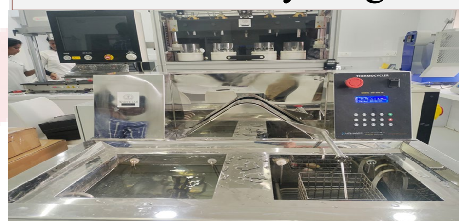
Samples prepared for thermocycling
