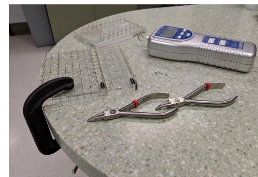
Fig. 3 Acrylic block jig holding elastics apart at a length of 3x ID
