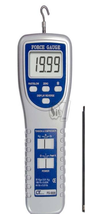
Fig. 4 Lutron Fg 5005 gauge for force measurement
